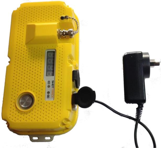
Charging is accomplished by plugging a standard 12-volt plug pack into the right hand rear socket.
