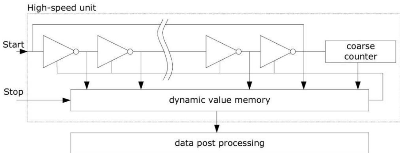
An output pulse is generated by the high speed field programmable gate array device which is injected into the cable. After a precise “guard time interval” the Time to Digital Converter is supplied with a start pulse. The detector circuit then produces a “stop” pulse when the original injected pulse is reflected from either an open or short circuit back to the unit. This “stop pulse” halts the Time to Digital Converter and the time elapsed is saved.
