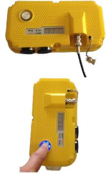
*If after reading the triggered data, the unit detects that the cable has returned to its original length then the unit will RE-SET itself assuming a transient trigger condition has falsely triggered the unit (for example a truck running over the cable)*
